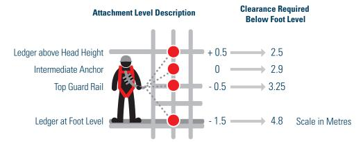
When attaching to Scaffold always check the integrity of the anchorage point you intend to use. In the case of system scaffold you should ensure the selected anchorage point is approved for use by the manufacturer.
